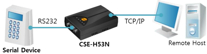
Figure 1-1 1:1 connection with a PC
