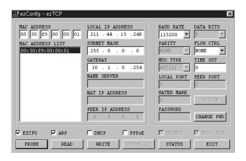
Run HotFlash to enter IP address in the IP address window according to ezConfig. The following picture shows the IP address, which is set to 211.44.13.248:
