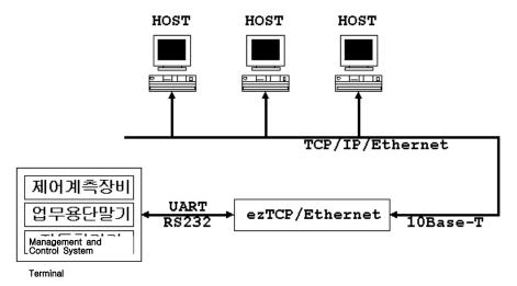
If of instrument liter (hereafter a host) is connected to the TCP port of ezTCP over an Ethernet network, the serial port of the DTE is connected virtually to the TCP port of the host. Then, ezTCP will function as an intermediate device between the serial port and the TCP port.
